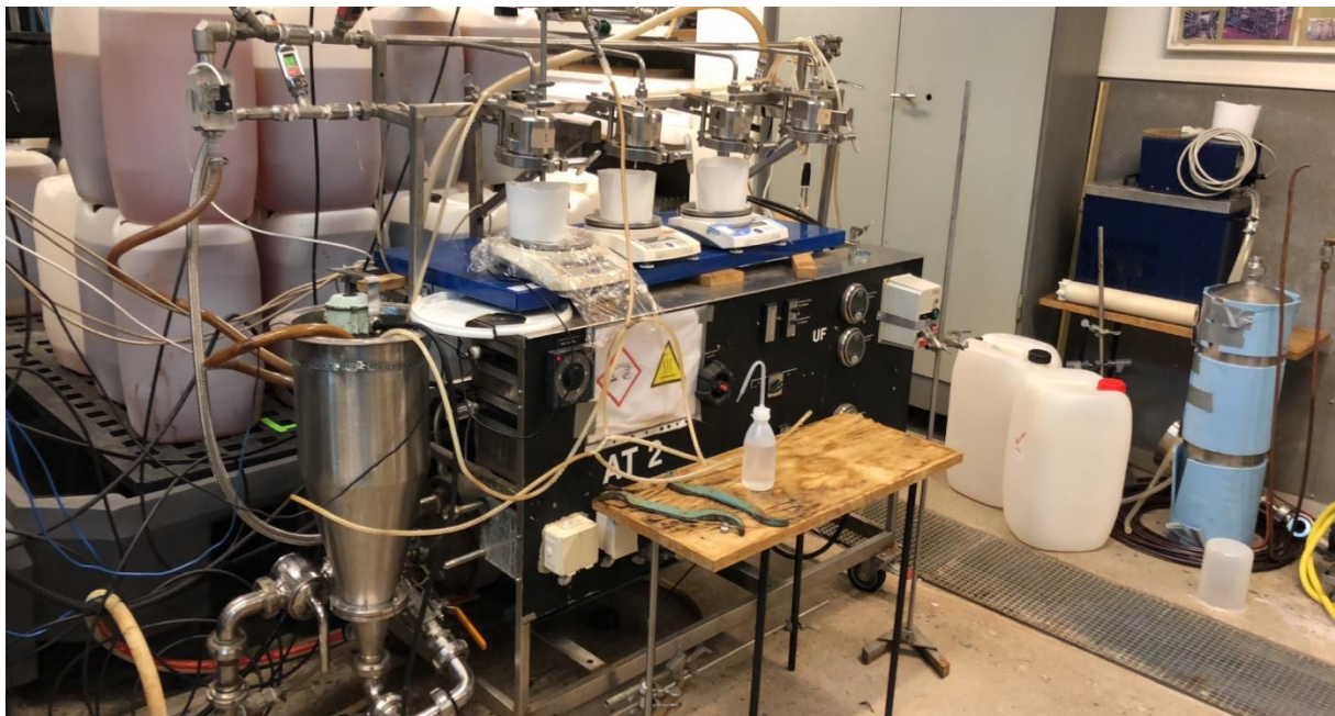
Figure 6 Photo of the equipment used in LTH to perform RO experiment.
