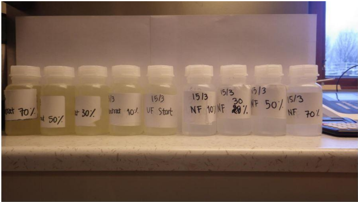
Figure 7. The picture shows the nanofiltration results at different VR from the fourth batch. In the middle is the UF permeate, on the right is NF permeate and on the left is NF concentrate.
