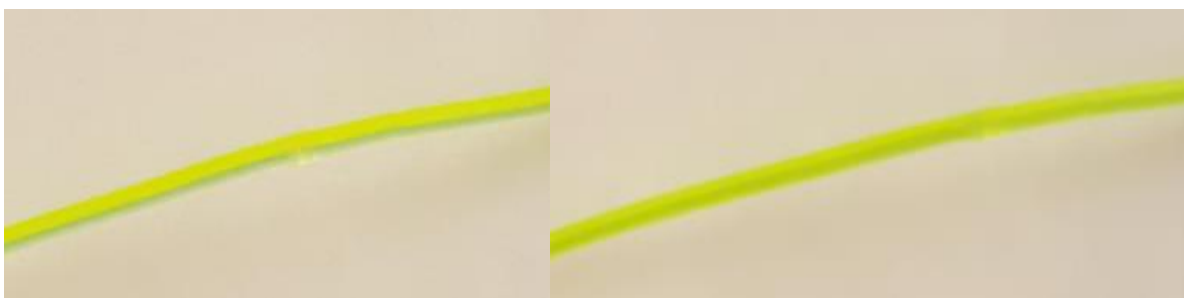
Figure 43: Left figure show fluid segregation at flowrate 1ml/min compared with apparent complete mixing at 10 ml/min for mix ratio of 50%.
