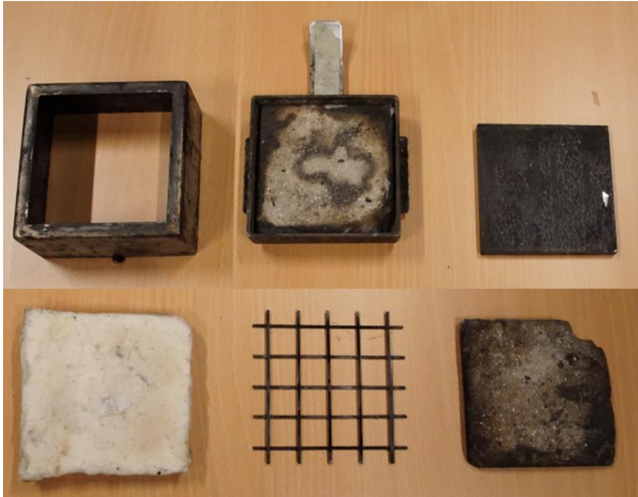
Figure 16 – Components of the specimen holder
