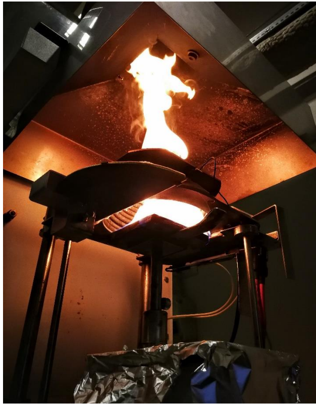
Figure 23 - Shell DIALA oil, burning process
