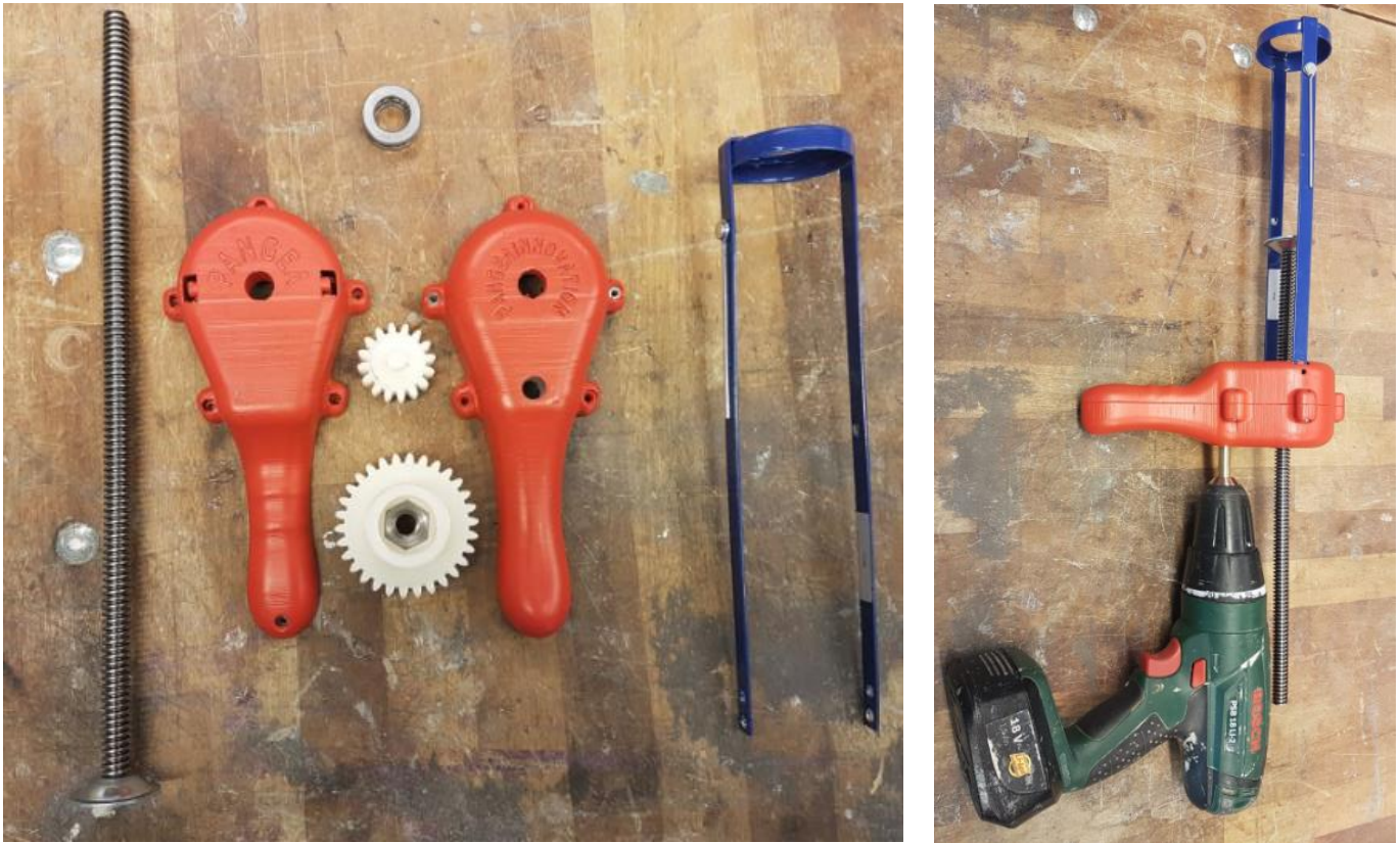
Figure 2.28 All components disassembled to the left and assembled to the right
