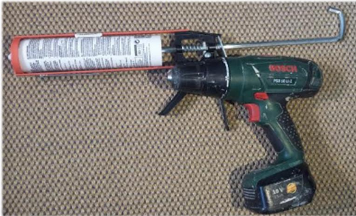
Figure 2.7 The placement of the caulking gun relative to the electric drill. Leadscrew will move above electrical drill as illustrated.
