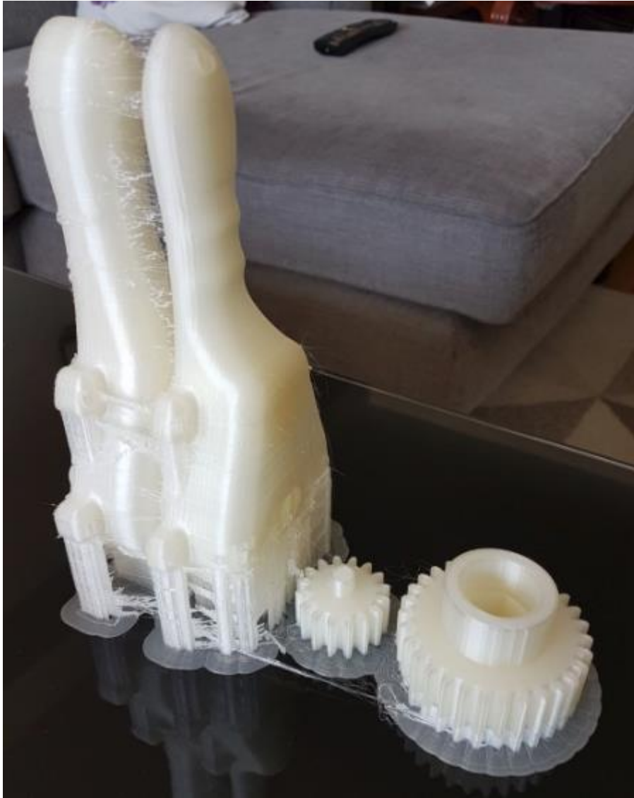
Figure 2.26 The 3D printed parts. Housing and gears.
