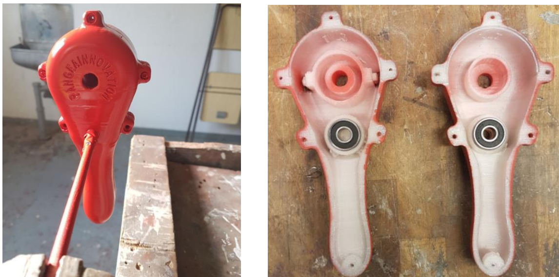
Figure 2.29 The colored housing to the left and the inside of the housing to the right with bearings assembled
