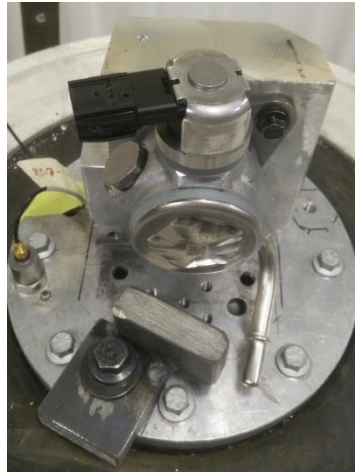
Figure 24, HPFP mounted to the fixture in Z-direction.
