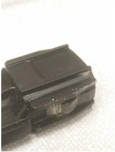
Figure 66: 700 Hz connector wear.
