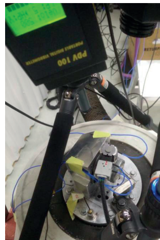
Figure 29: Lasers pointing at holes
