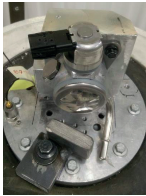
Figure 24, HPFP mounted to the fixture in Z-direction.
