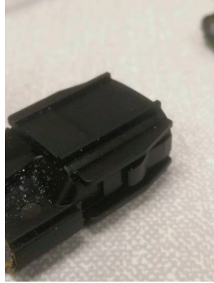
Figure 67: 800 Hz connector wear.
