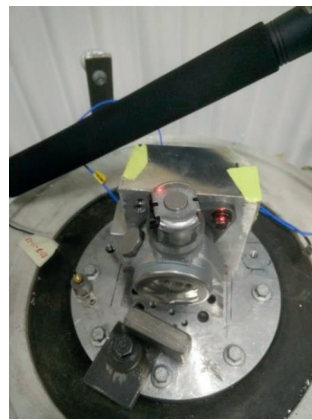
Figure 57: Fuel connector removed
