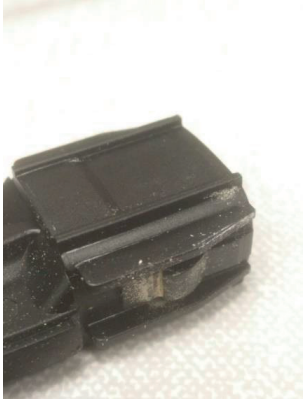
Figure 66: 700 Hz connector wear.
