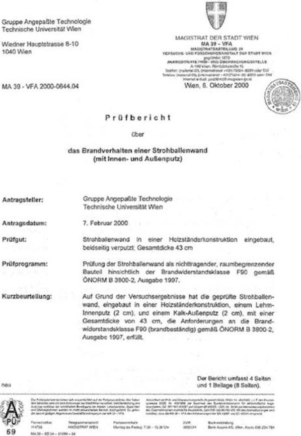
Figure 40. F90 fire test result of a clay rendered straw bale wall with wooden studs. (Source: Gruber, 2018)
