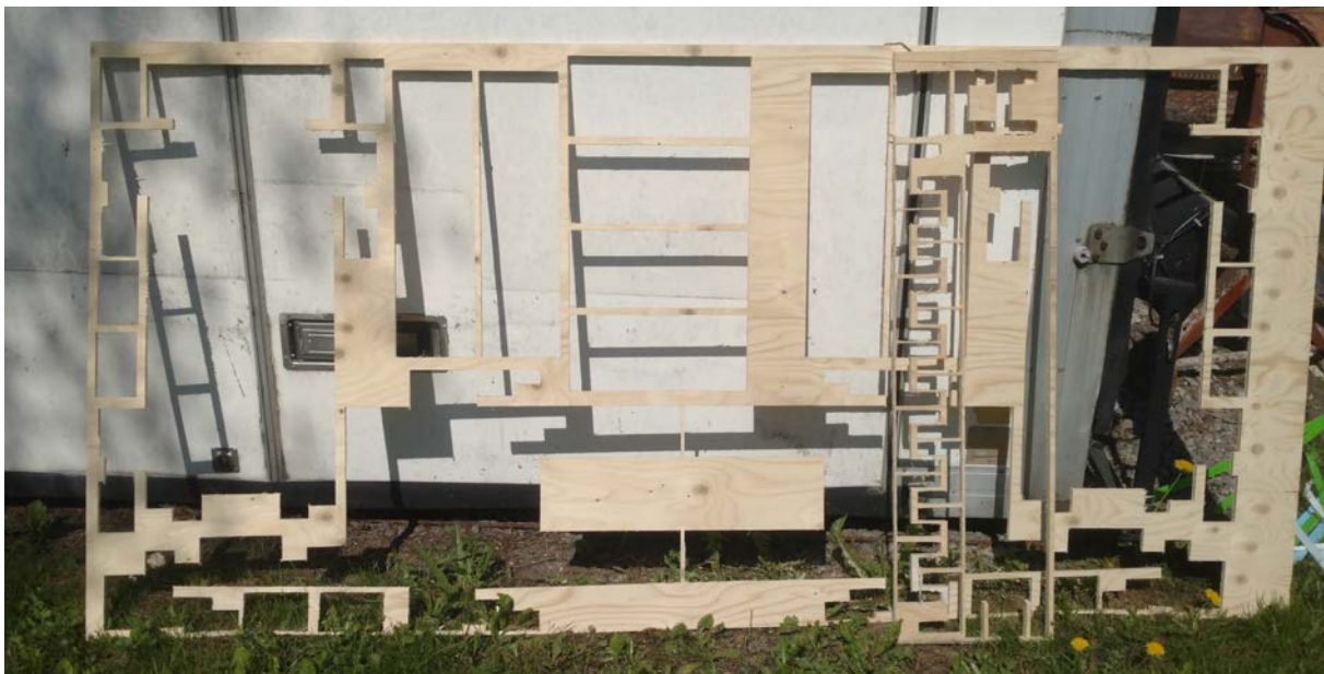
Figure 6. Waste after CNC cutting of the prototype, May 2018, Vitaby, Skåne, Sweden (Photo: Author)
