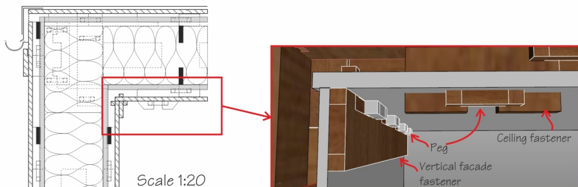
Figure 14. An example of the reversible connection of ceiling and inner façade elements.
