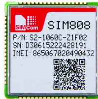
Figure 4.6: The SIM808 module with GPS positioning and GPRS mobile communication.
