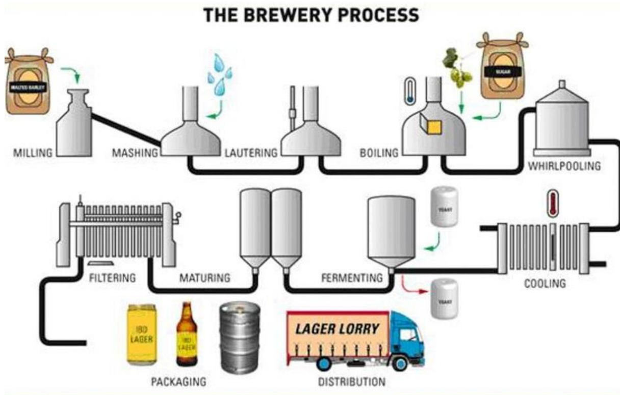
Figure 2-1. A schematic chart of the beer brewing process not including the malting step (ABC News, 2018).
