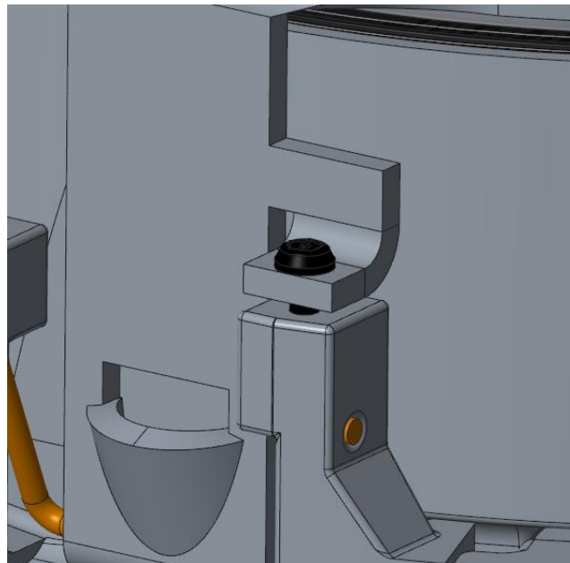
Figure 8.4 Pocket for opening the lock and a safety screw from lock to bracket towers
