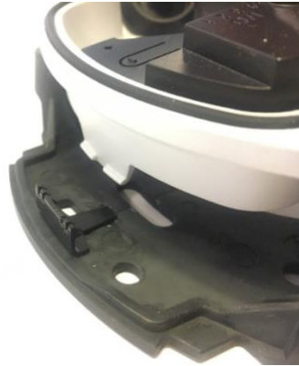
Figure 3.7 Plastic clip attached to aluminum bracket
