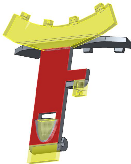
Figure 8.1 Flat pattern of the sheet metal lock in Creo Manufacturing
