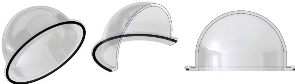
Figure 9.6 Dome with gasket pre-assembled. Middle and right: Cross section showing the track on top of the flange and the placement of gasket around wall under the flange
