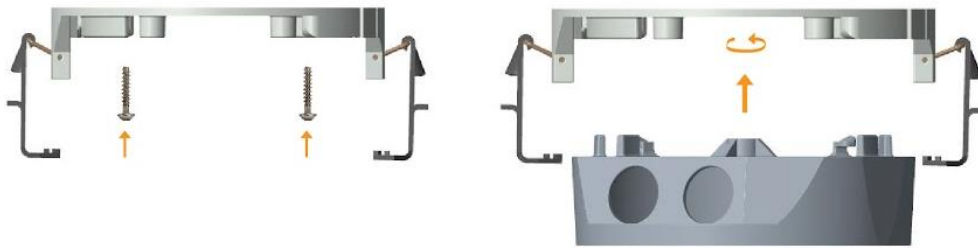
Figure 9.7 Left: mounting the bracket in the ceiling with screws, locks hanging vertically due to gravity. Right: Placing the chassis on bracket
