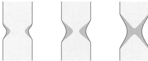
Figure 2.12: A schematic representation of the formation of necking in a thin sheet [10].
