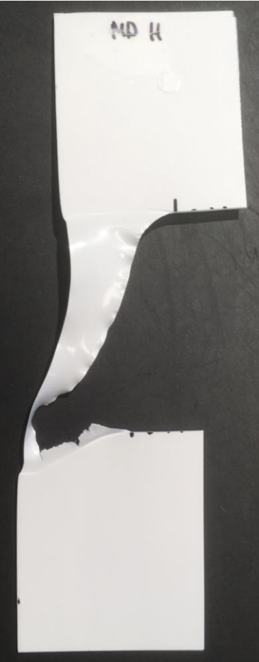
Figure 3.15: Fractured MD sample. Black vertical line indicate original crack edge.
