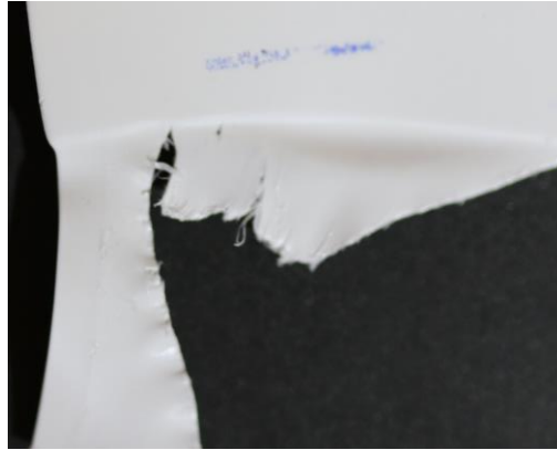
Figure 3.19: Section of fractured MD sample studied in SEM.
