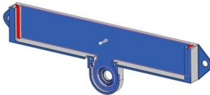
Figure 8.34: The front of the shell with the undercut analysis.
