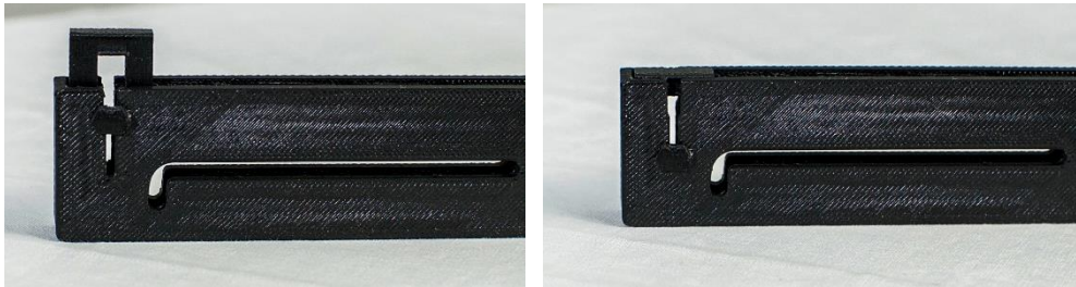
Figure 6.9: Photo of concept D when the guide is extended (left) and when the guide is hidden (right).
