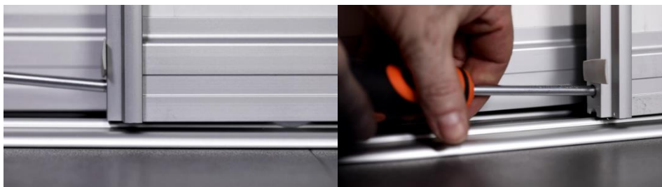
Figure 5.17: Fastening the door [21].
