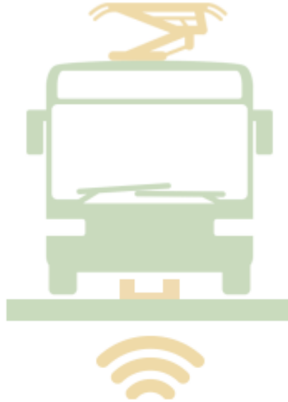
Figure 1.3: The three main ERS strategies marked in yellow. Conductive charging from roof receiver or road rails and inductive charging through the road.
