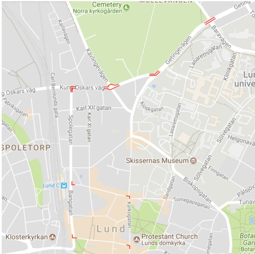
Figure 6.4: Several obstacles are chosen and added to ensure full charging coverage for each bus line. The total unavailable distance is 500 meters which gives approximately 10 kWh extra charging marginal input to the algorithm.
