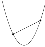
Figure 2.3 The graph of a convex function ( f(x) = x^2 ). Note that a line segment between two points of the graph lies above the graph of the function.
