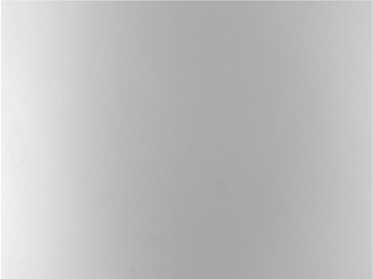
Figure 7: An image taken of a 50% Spectralon reflectance panel during the manual radiometric calibration in the Green band where vignetting can be seen. The image taken is part of the dataset used to derive the vignetting statistics. The image taken was done during radiometric calibration using a 50% spectralon reflectance plate. The green band was chosen as of visualization purposes.
