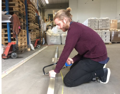
Figure 6.12 Cutting aluminium pipe.
