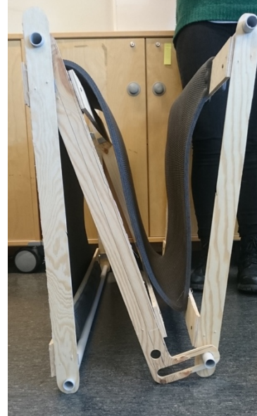
Figure 5.25 Model of the Hockey stick concept while folded.
