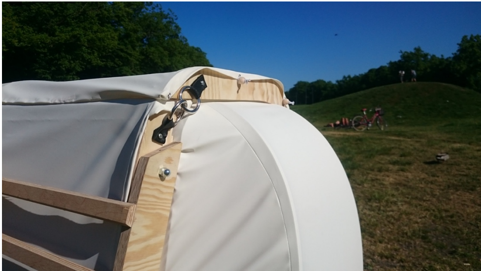
Figure 7.13 Two rings locking the sides together during cycling.
