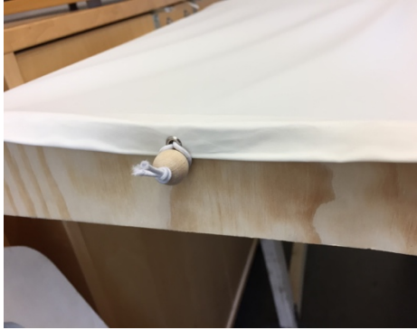
Figure 6.72 Elastic bands and wooden balls laced through eyelets in the fabric.
