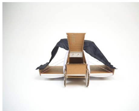
Figure 5.44 Cardboard model of Teardrop chuck trailer with pulley mechanism in scale 1:5 in unfolded position.
