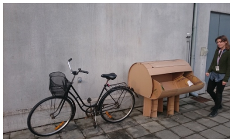
Figure 5.17 Barrel concept in scale 1:1 with open luggage area.
