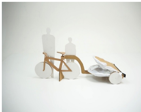
Figure 5.5 Bellow concept in folded position in scale 1:5.
