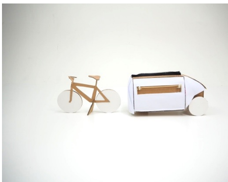
Figure 5.43 Cardboard model of Teardrop chuck trailer with pulley mechanism in scale 1:5 in folded position.
