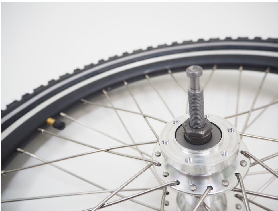
Figure 6.34 The stub axle mounted in the wheel.
