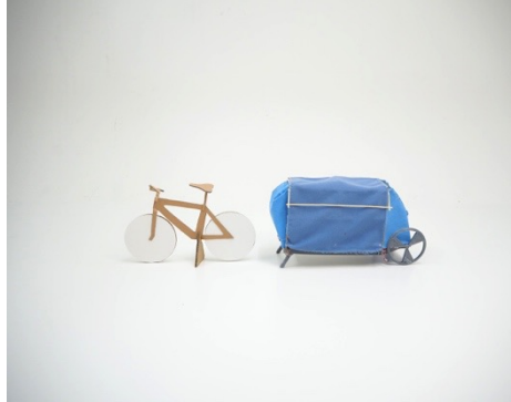
Figure 5.45 Detailed cardboard model in folded position in scale 1:5.
