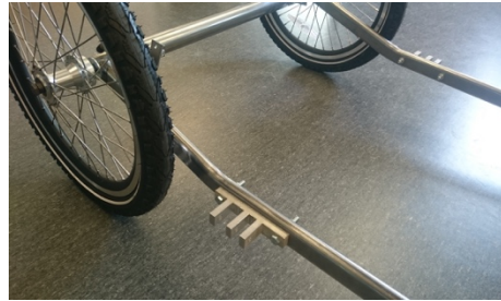
Figure 6.44 Water cut ears assembled to the steel chassis.
