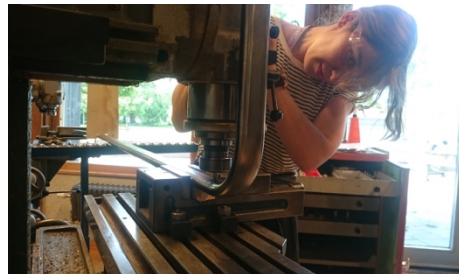
Figure 6.28 Drilling in chassis.
