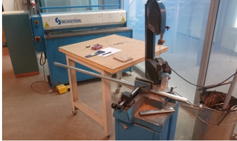
Figure 6.50 Sawing the pipe into legs.
