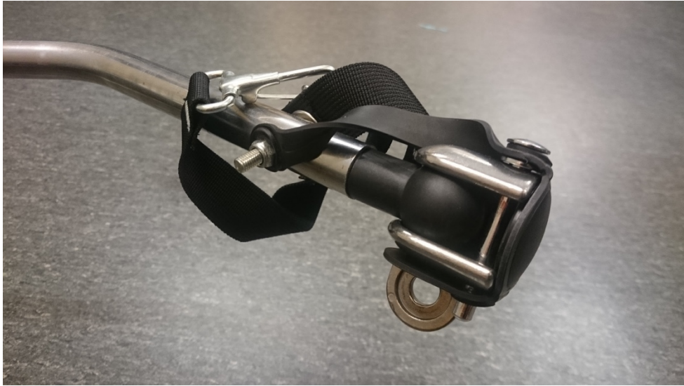
Figure 6.54 Components sponsored by Thule mounted in the projects custom made hitch arm.
