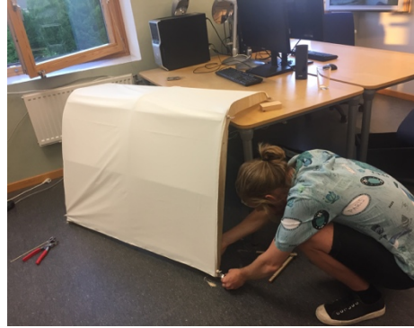
Figure 6.73 Attachment of fabric onto the wooden skeleton.
