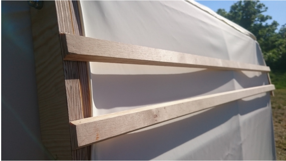
Figure 7.12 The outer legs also acting as handles to open the camper.
