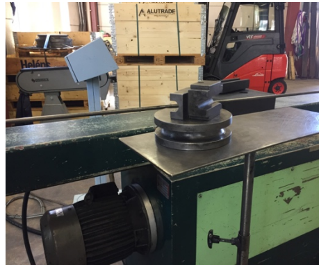
Figure 6.26 The tool used for bending the steel chassis.
