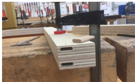
Figure 6.60 DOMINO joining method.
