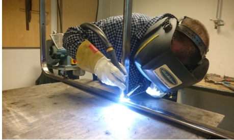
Figure 6.29 Welding done by Bert in the IKDC workshop.
