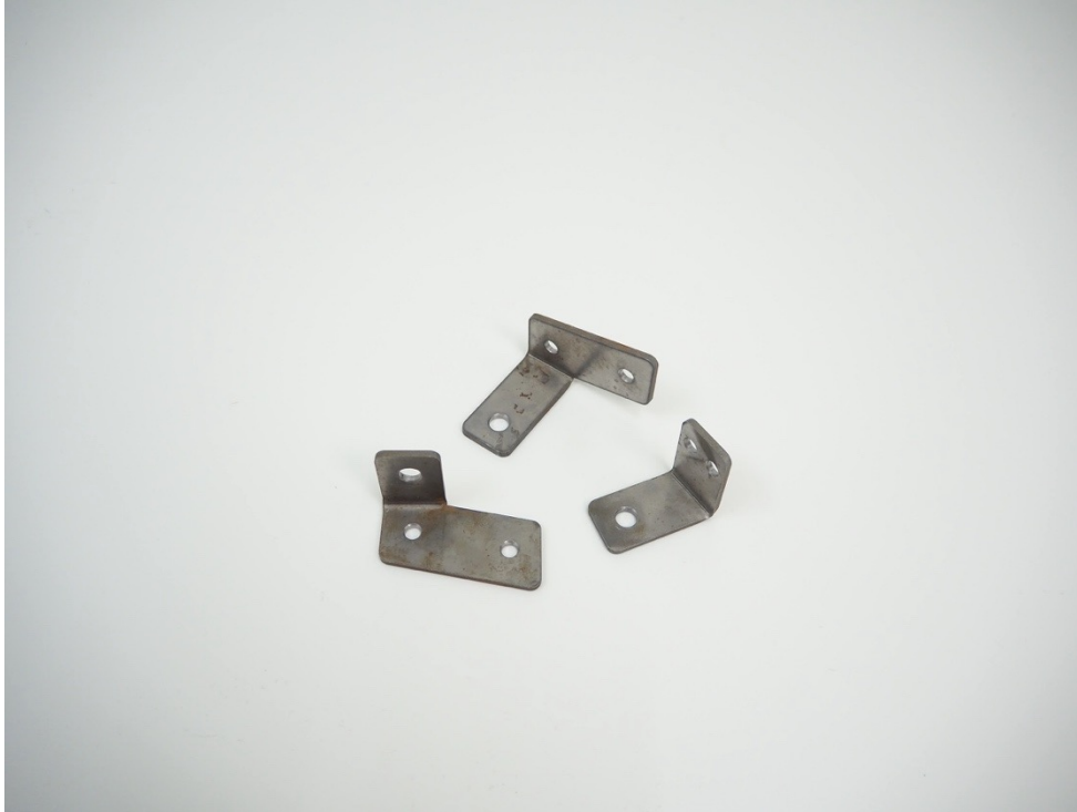
Figure 6.49 Three types of angle brackets after water cutting and bending.
