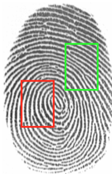
Figure 1.5: Overlap between a verification template (green) and an enrollment template (red) captured by a small sensor. Original fingerprint image from [1, p. 131].
