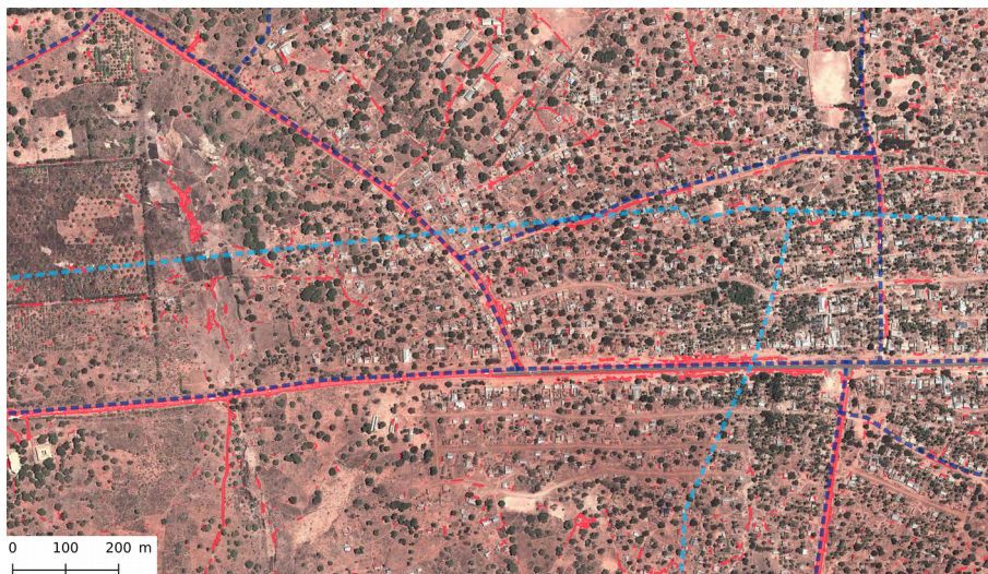
Figure 10c. Visualisation of the road network extracted in study area C from high-resolution Google Earth imagery using the method described in Ojo et al. (2016). In orange/red are the extracted road network. The gROADS road network is shown in light blue and the OSM road network is shown in dark blue. The satellite imagery used for extraction and validation is set as the background and is provided by Google, Airbus DigitalGlobe.
