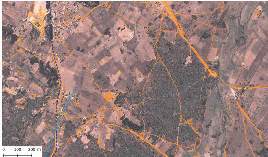
Figure 10b. Visualisation of the road network extracted in study area B from high-resolution Google Earth imagery using the method described in Ojo et al. (2016). In orange/red are the extracted road network. The gROADS road network is shown in light blue and the OSM road network is shown in dark blue. The satellite imagery used for extraction and validation is set as the background and is provided by Google, Airbus DigitalGlobe.
