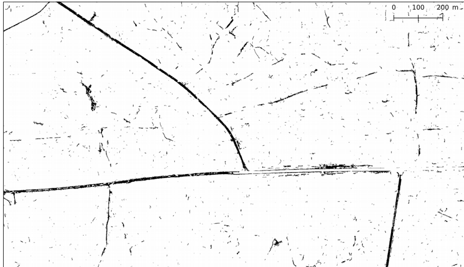
Figure 9c. Binary visualisations of the road networks extracted in study area C in Tanzania from high-resolution Google Earth imagery using a method described in Ojo et al. (2016). Black pixels represent roads; white pixels represent non-roads.
