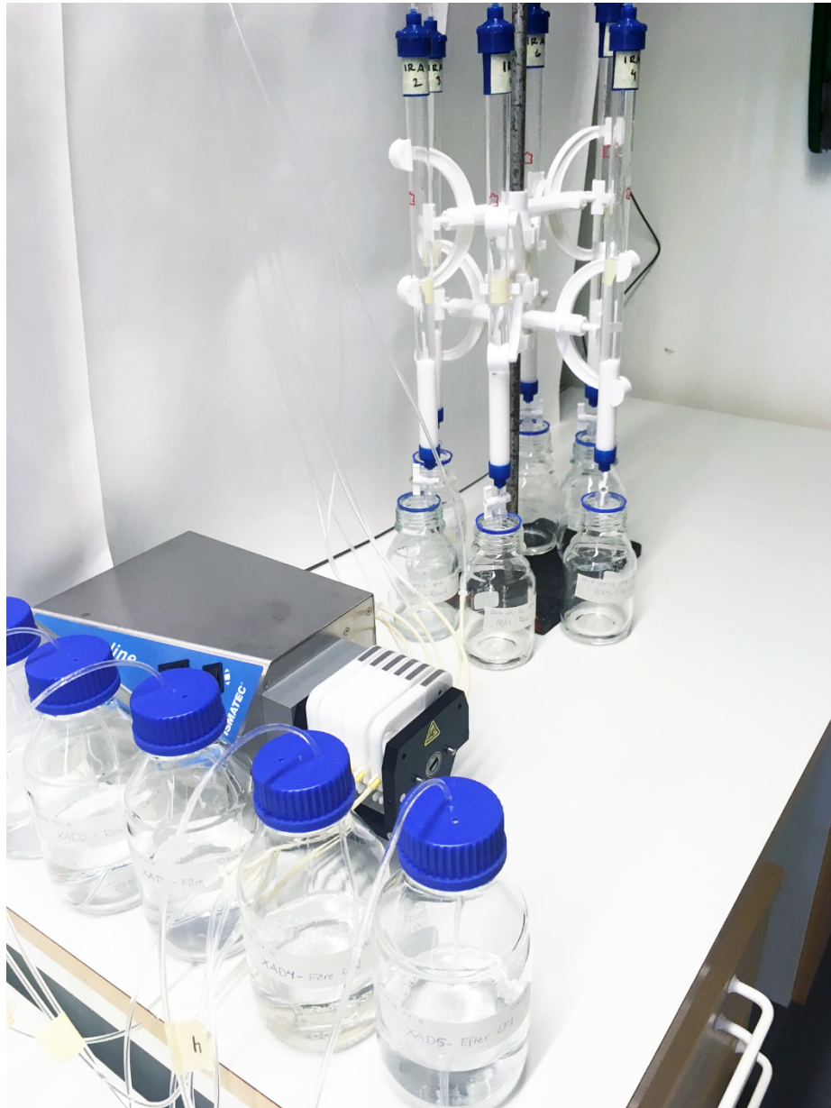
Figure 5. The laboratory setup when fractionating through the IRA columns. In the front: glass bottles with water samples, in this case from effluent from the previous XAD columns. In the middle: the pump that pumps water from the bottles to the IRA columns. In the back: the IRA columns and the effluent water that is collected in glass bottles.
