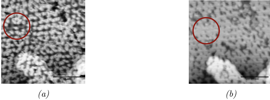
Figure 4: Comparison of two different charge density contours of the same location in the sample. Scanned surface: Boron Nitride deposited on Gr/Ir(111) with electron assisted growth and annealed at 1323 K. a) The graphene substrate is visible underneath the adsorbates (red circle). b) Due to a change on the morphology of the tip, the graphene is not visible anymore.
