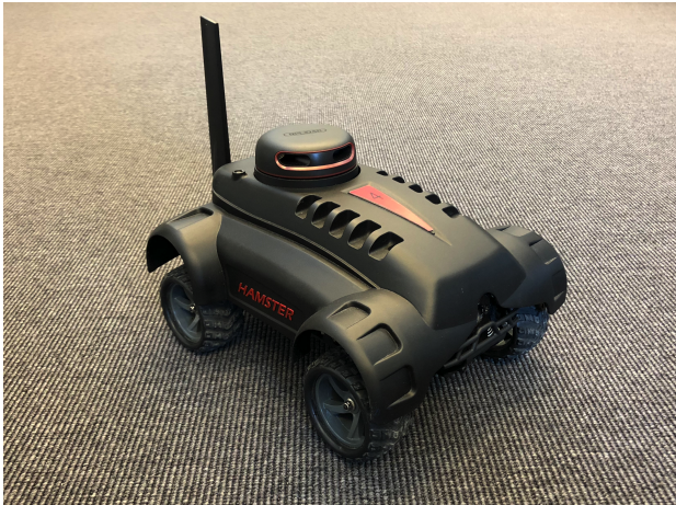
Figure 6.1 Picture of the HamsterV5, the vehicle platform used for driving experiments.
