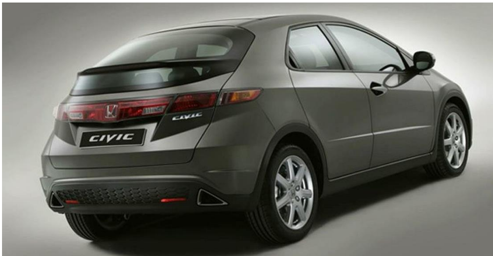
Figure 4.6 – Honda civic merged backlite and spoiler [25]
