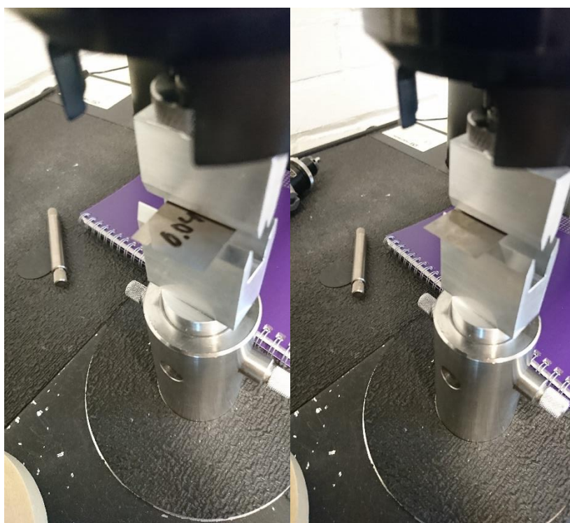
Figure 19 The picture to the left shows the centered position of the sample and the picture to the right shows the off centered sample position.
