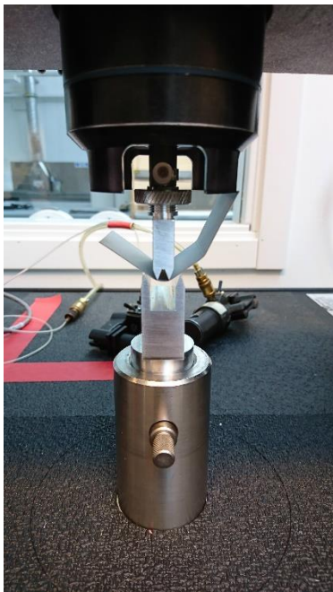
Figure 58 The samples interfering with the load cell during the measurement of the uncreased value.
