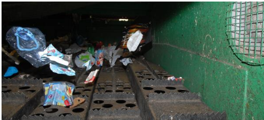
Figure 31 – Ballistic separator, ValorSul 2018c
