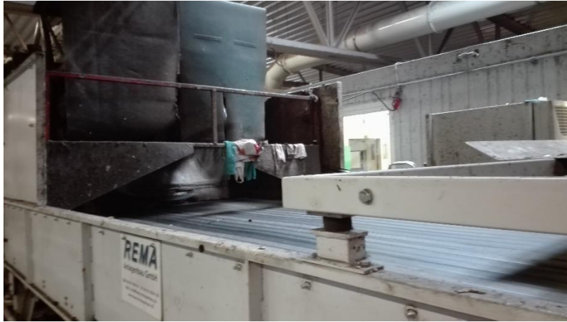
Figure 23 – Machine that separates tapes from the plastic packaging waste stream
