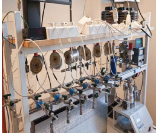
Figure 5: Picture of the conventional graphitization apparatus. Picture taken from: E Andersson Georgiadou: Exploring the possibilities of ^{14}\text{C} bomb-pulse dating of human tissue samples. Doctoral dissertation. Lund University, 2014.
