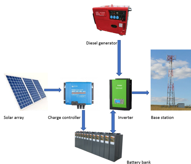
Figure 5.13: Solar diesel hybrid site set up
