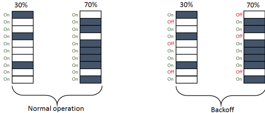
Figure 4.1: Overview of an example with 10 resource blocks in frequency domain. In normal operation all PAs are biased, showed as "On" in the image. With backoff to the right there is a limit on the number of biased PAs and some are unbiased, showed as "Off". In this example the throughput is limited to 70% of its original value. This backoff can be used as an ECO-mode.
