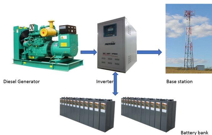
Figure 5.12: Fully diesel powered site set up
