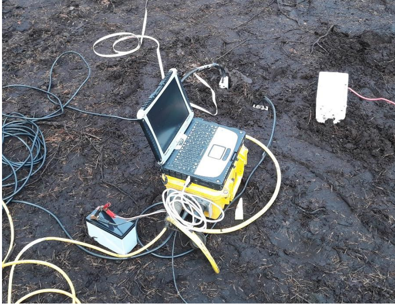
Figure 3.2: Seismograph system, setup from Ageröds mosse.
