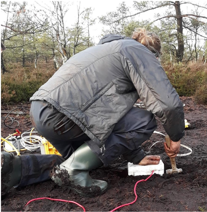
Figure 3.5: A sledgehammer used as the source in the small-scale investigation at Ageröds mosse.
