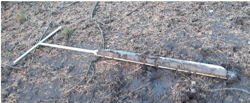
Figure 3.1: The Russian sampler used with peat in the steel chamber.
