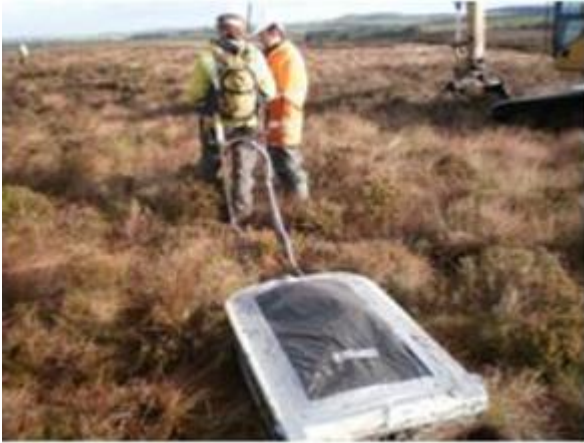
Figure 4.3: GPR used in field work at a peat bog (Trafford & Long 2016).
