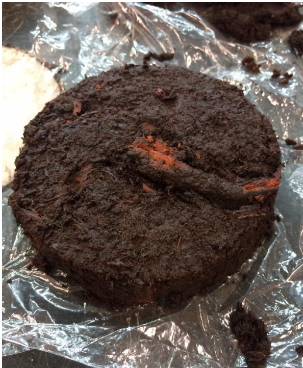
Figure 2.5: Timber fragment illustrating the heterogeneity of peat.
