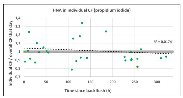
Figure 10: Bacterial counts in effluent carbon filter water, individual carbon filters compared to the average that date. The individual filter count is divided by the average, giving a ratio used for the Y-axis. Each dot is a mean value of triplicates.  $R^2$  values are presented in each graph.
