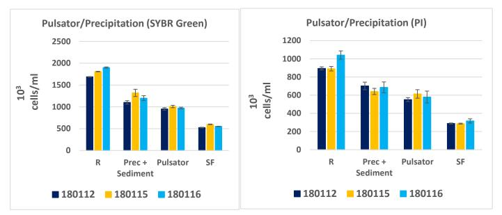
Figure 11: Bacterial separation efficiency of the two flocculation steps and sand filtration. Total and intact cell counts for treatment steps Precipitation + Sedimentation and Pulsator compared to before (R) and after sand filtration.
