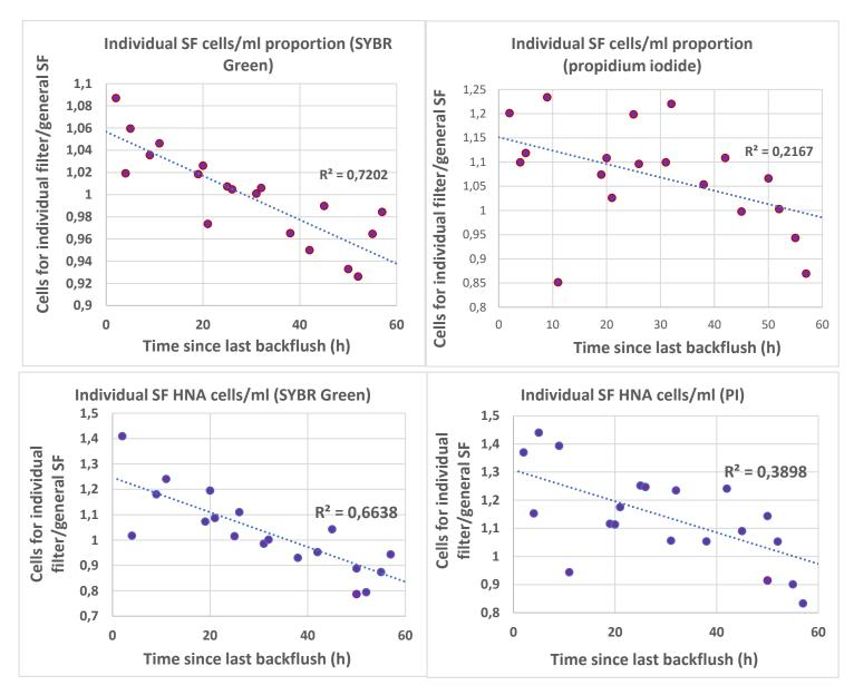
Figure 9: Bacterial counts in effluent sand filter water; individual sand filters compared to the average that specific date. The individual filter count is divided by the average, giving a ratio used for the Y-axis. Each dot is a mean value of triplicates.  $R^2$  values are presented in each graph.
