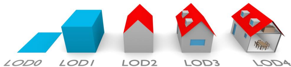
Figure 5 Building represented in CityGML LoDs (Biljecki et al. , 2014), licensed under Creative Common 4.0
