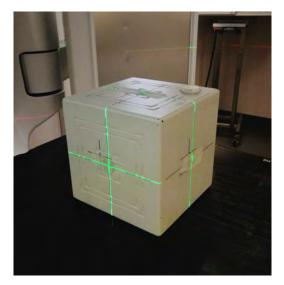
Figure 4: The QUASAR<sup>TM</sup> Penta-Guide Phantom used for the Routine QA.
