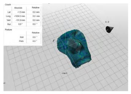
Figure 6: The live surface and the reference surface in perfect alignment, indicating a correct patient position.
