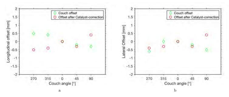
Figure 19: The isocenter offset (greeen markers) from couch angle 0° to couch angles 45°, 90°, 270° and 315° respectively in the longitudinal (a) and lateral (b) direction together with the offset after couch correction according to the OSS-indicated values (red markers). All values are presented according to the couch coordinate system, as position of the steel ball relative to the treatment isocenter.
