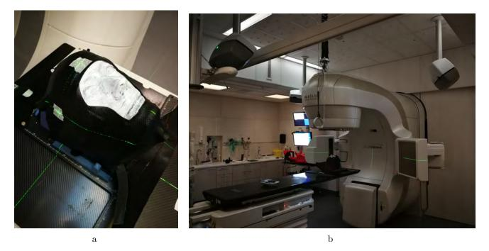
Figure 8: The Alderson RANDO Phantom immobilized with an open-face mask (a) and the treatment room with a Varian Truebeam linear accelerator and the ceiling-mounted three-camera OSS system (b).
