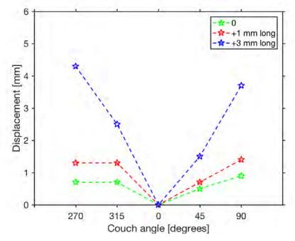
Figure 20: The magnitude of the total isocenter shifts indicated by the OSS system at couch angles  $\neq 0^{\circ}$ , with and without an intentional misalignment between the treatment isocenter and the OSS systems isocenter.
