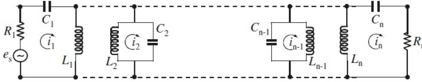
(a) Equivalent circuit of n -coupled resonators for loop-equation formulation.
