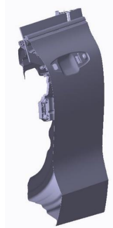
Figure 5.6 Cut front door, outer view
