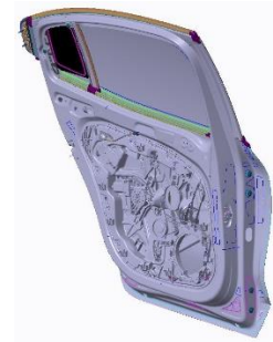
Figure 5.17 Rear door, side view.
