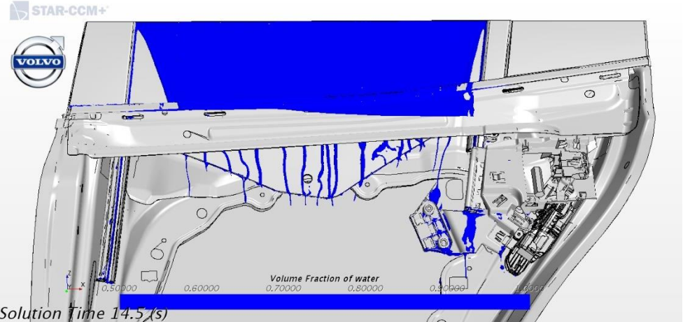
Figure 31 Water flow, front view
