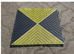
Fig. 2.1. GCP - Ground control point used in this project
