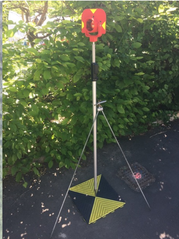
Fig. 4.4. Precise measuring of the position of a GCP.
