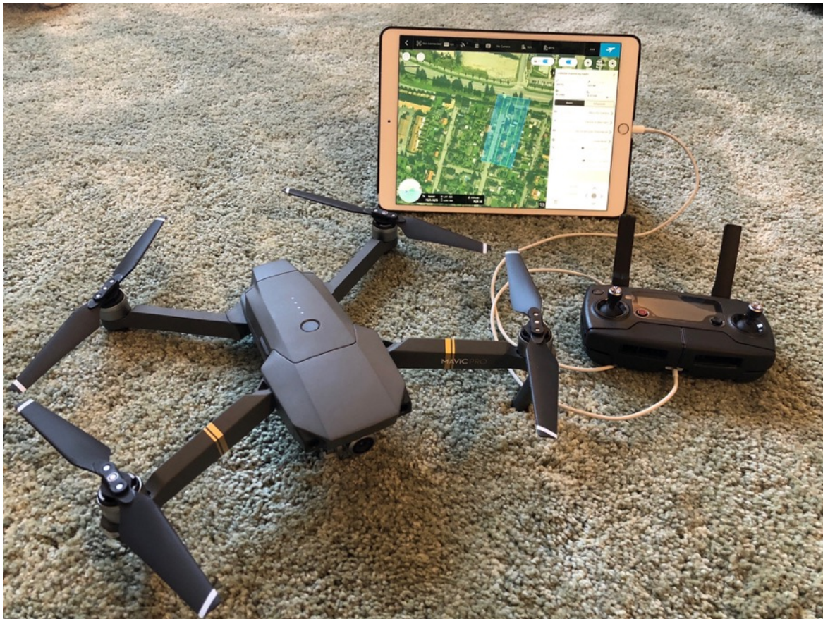
Fig. 3.2. The drone used in this thesis with its remote controller connected via USB cable to an iPad for telemetry data, flight planning and live video feed.
