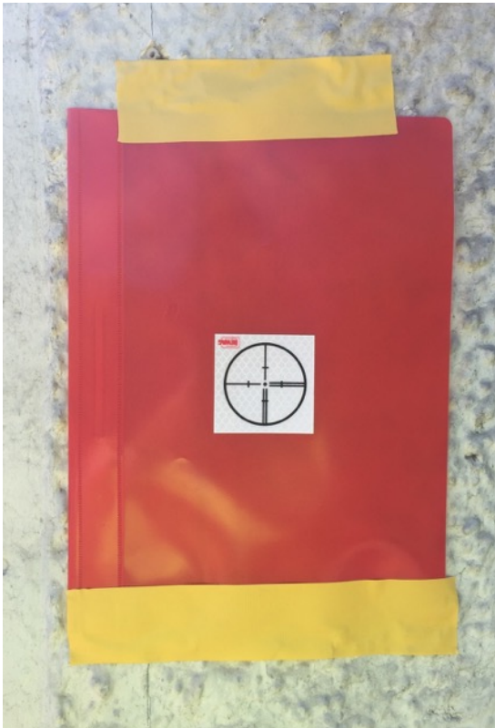
Fig. 4.3. Reflective target for total station measuring. The contrasting plastic sheet helps with later identification in the point cloud reconstruction phase.
