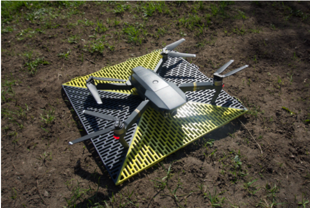
Fig. 4.8. One of the GCPs placed around the building.
