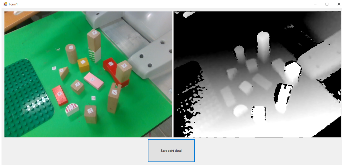
Figure 3.2: A screenshot of the point cloud capturer program. The left part of the window shows a live feed from the RGB camera, and the right part of the window shows a live feed from the depth camera, with closer points being more white than far away points.
