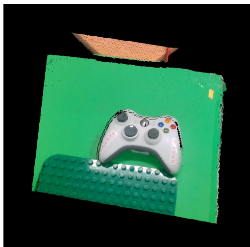
Figure 4.5: Original point cloud of the scene captured by the camera containing a wireless xbox controller.
