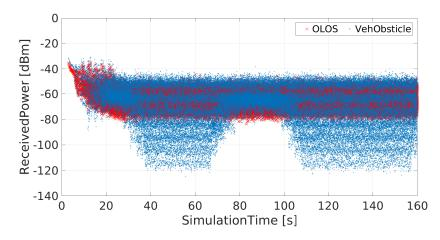
Figure 35: Comparison of Received Power, SingleSlopeOLOS and SingleSlope for LOS + Vehicle Attenuation
