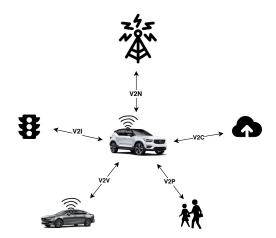
Figure 1: Communication of Vehicle with the surrounding such as Pedestrian (V2P), Vehicle (V2V), Infrastructure(V2I), Network(V2N) and Cloud (V2C)
