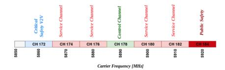
Figure 2: Channel types and spectrum in DSRC
