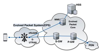
Figure 4: Structure of LTE
