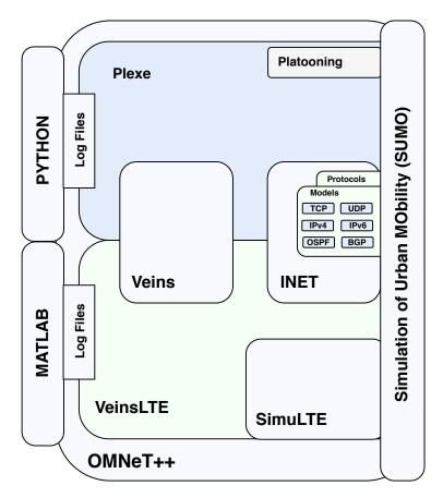
Figure 7: Relation among Plexe and VeinsLTE. Two independent frameworks VeinsLTE and Plexe that both use Veins and INET frameworks. The difference is that Plexe contains Platooning features while VeinsLTE contains the stack of LTE.
