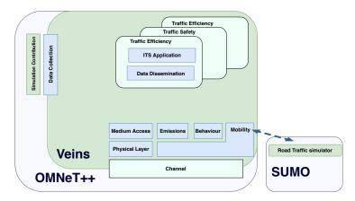
Figure 8: Architecture of Veins, source: [11].
