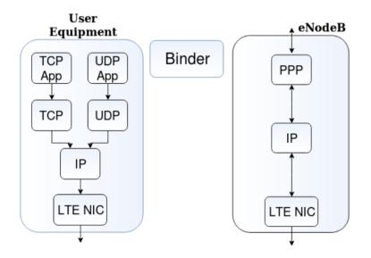
Figure 9: Architecture of simuLTE, source: [15].
