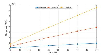
Figure 40: Throughput for DSRC in Highway Scenario
