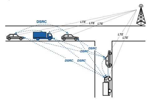
Figure 16: Simulation setup scenario for DSRC and LTE
