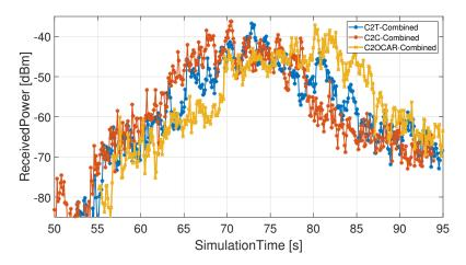
Figure 21: Average received power over simulation time using the combined model for communication in Yngve Scenario. Rx vehicle is in the group 1 white car from Fig.20 and TX is all vehicles in the group 2: yellow Car, yellow Truck, lightblue OCar.
