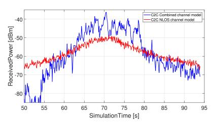
Figure 22: Yngve intersection, One Link communication C2C through Combined model and NLOS model.
