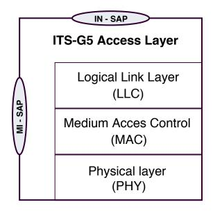
Figure 3: Architecture of ITS-G5, source: [10]
