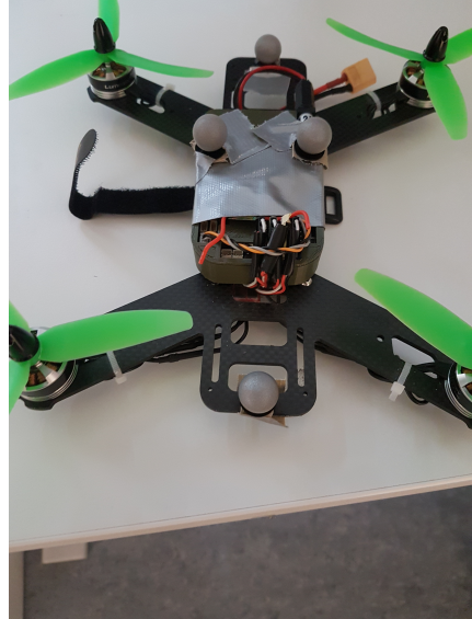
A quadcopter equipped with reflective balls for camera detection.
