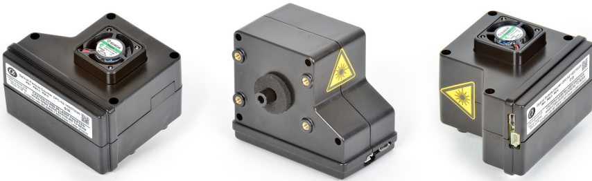
Figure 8: The Alphasense OPC-N2. The dimension of the sensor is about 70 x 65 x 60 mm.
