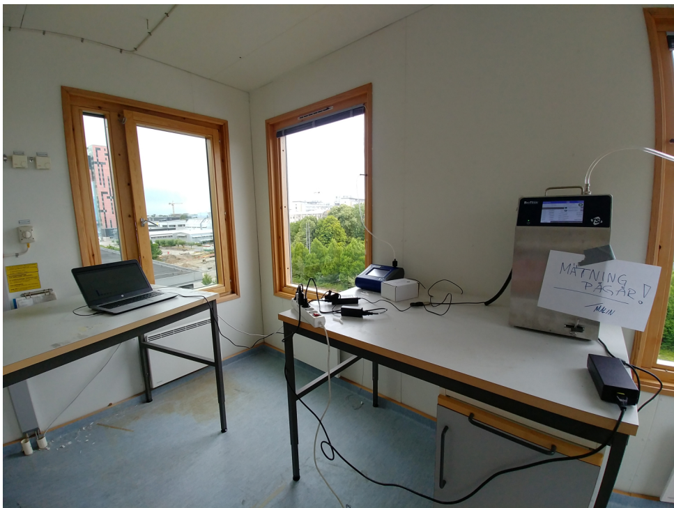
Figure 31: The measurement setup during the first experiment. The OPC-N2 was taking in air through an opening in the window to the left.
