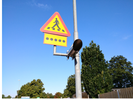
Figure 27: The purpose of the reflector is to reflect the light from the light source to the photodetector. This reflector is 50 m away from the light source, which gives a total distance of 100 m.
