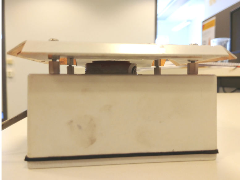
Figure 20: The side-view of the box with the NO 2 -B43F sensor installed. The lid of the enclosure is faced downwards.
