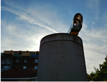
Figure 26: Light source of the DOAS. The light is created from a tungsten tip. In the same unit is the photodetector to receive the light from the reflector.
