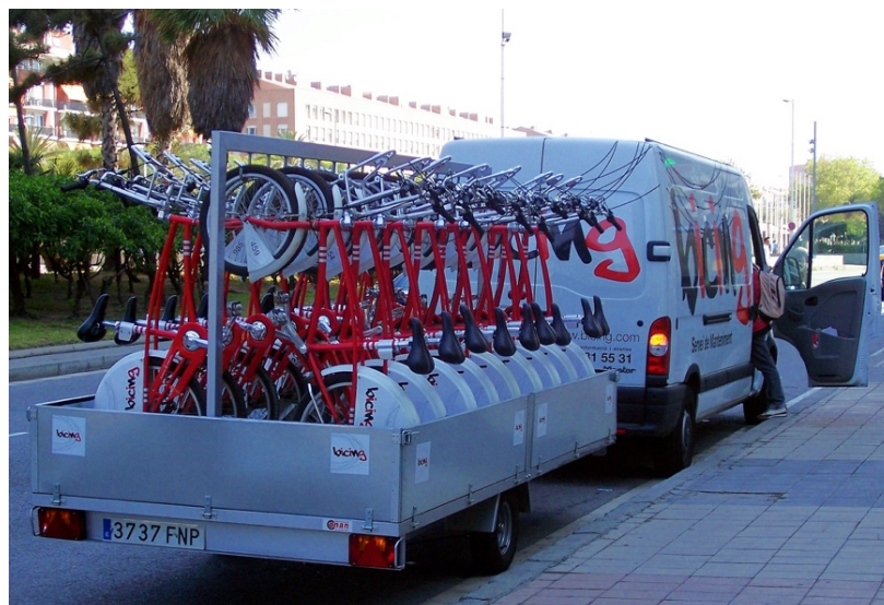
Figure 5-2. Bicing redistribution truck
