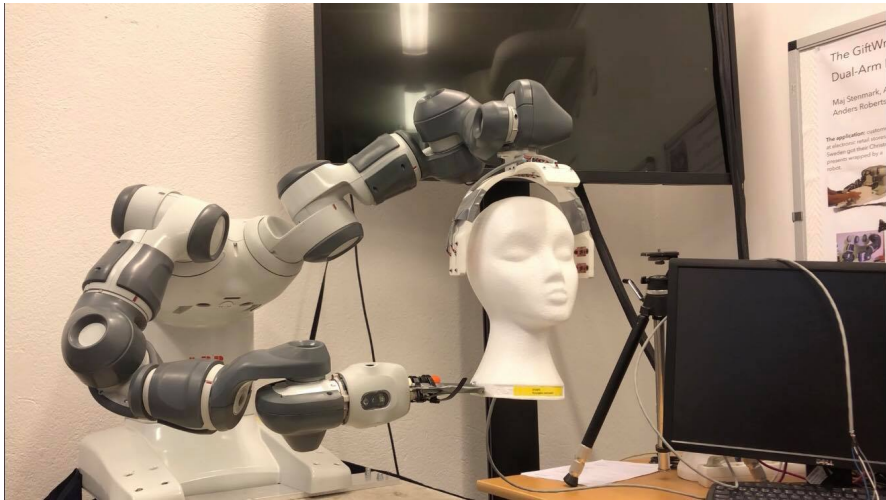
Figure 3.3 The head and platform mounted on the robot.
