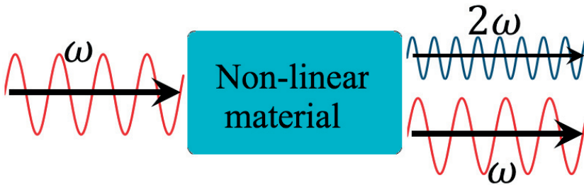
Figure 10.9: The Second Harmonic Generation (SHG) conversion in a nonlinear material [16]
