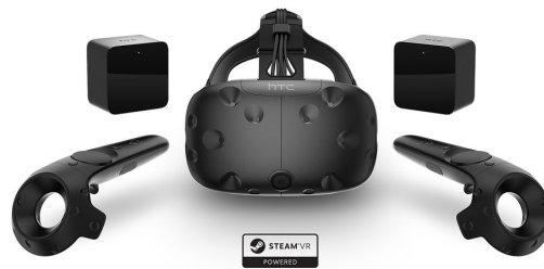
Figure 2.2: The HTC Vive, showing the HMD, hand controllers and lighthouse beacons.
