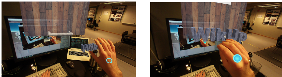
Figure 5.3: This showcases the built-in indicator for when a grab is possible: a blue donut shape appears at the back of one's hand. When grabbed the donut is filled in and becomes a full blue circle. When released, the circle becomes a donut again, and when out of reach (outside the collider) the donut disappears.
