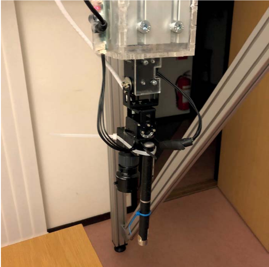
Figure 16: The final construction of the spray nozzle setup
