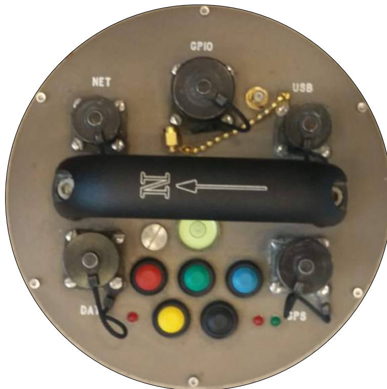
Figure 4.7: A seismometer seen from above, Photograph: Adam Cederquist
