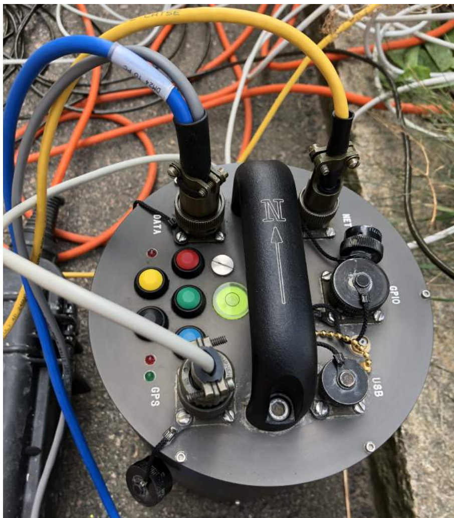
Figure 4.8: A Seismometer with all cables connected, Photograph: Juan Negreira
