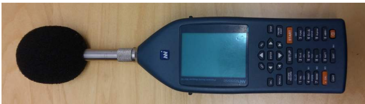
Figure 4.10: A sonometer used in the measurements, Photograph: Adam Cederquist
