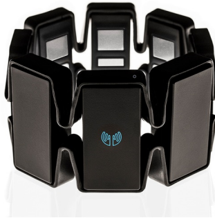
Figure 3.1: The Myo Armband used to collect sEMG data. Source: Thalmic Labs/Myo
