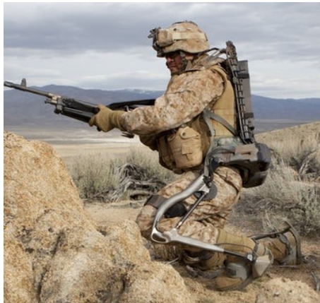
Figure 2.1: Lockheed Martin's HULC exoskeleton. The batteries and some mechanics are worn as a backpack.
