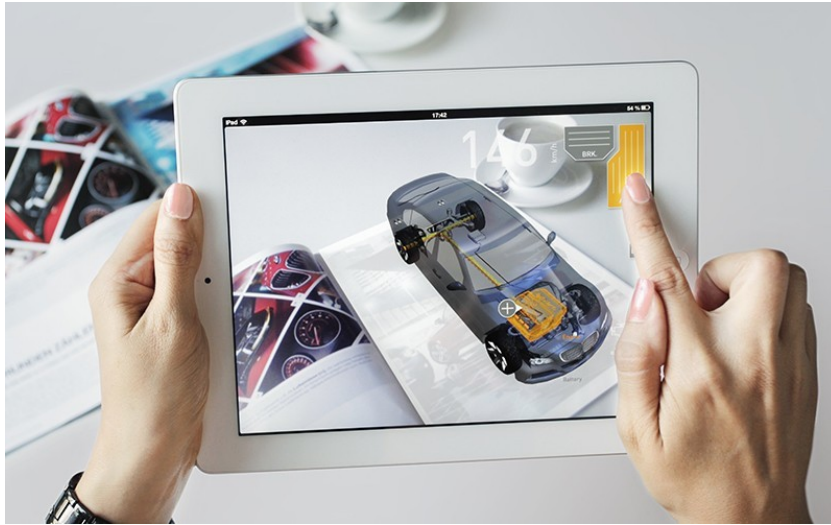
Figure 3.1: A virtual object in the form of a car being rendered on top of a marker in a magazine.
