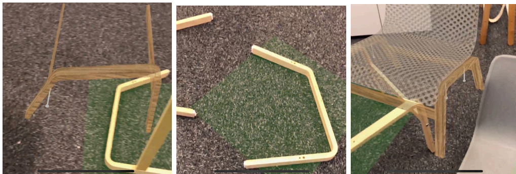
Figure 8.5: Images from the application when having started the ARScene, finding objects and showing animations when putting them together. The green rectangle on the floor is an indication that the part has been recognized by the application. We call these markings.
