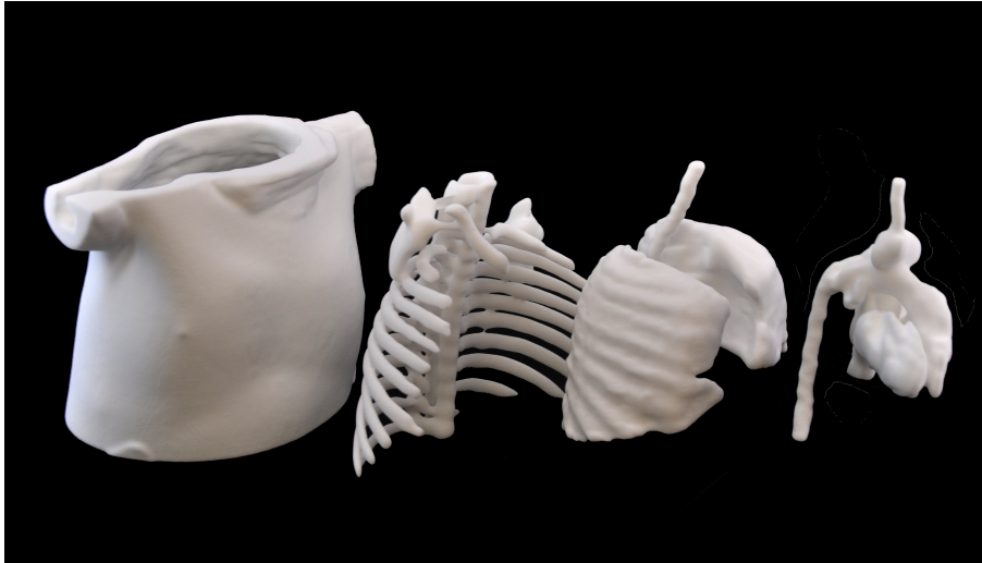
Figure 9: The 3D printed model of a prematurely born baby torso used for realistic measurements of oxygen concentration in the lungs. From the left is an outer body, hollow, to be filled with fat and muscle phantom, bone structure, solid, lungs, hollow, containing air and the heart, hollow, to be filled with heart muscle phantom.
