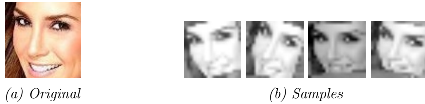
Figure 3.3: Multiple samples were created from the original by applying geometric transformations and pasting it onto random negative images. The samples were also rescaled and converted to greyscale.
