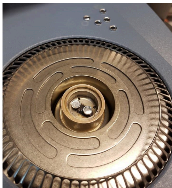
(b) The reference pan(upper left) and the sample pan(bottom right).
