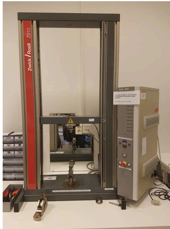
Figure 3.12: The Zwick/Roell Z010 tensile testing apparatus.
