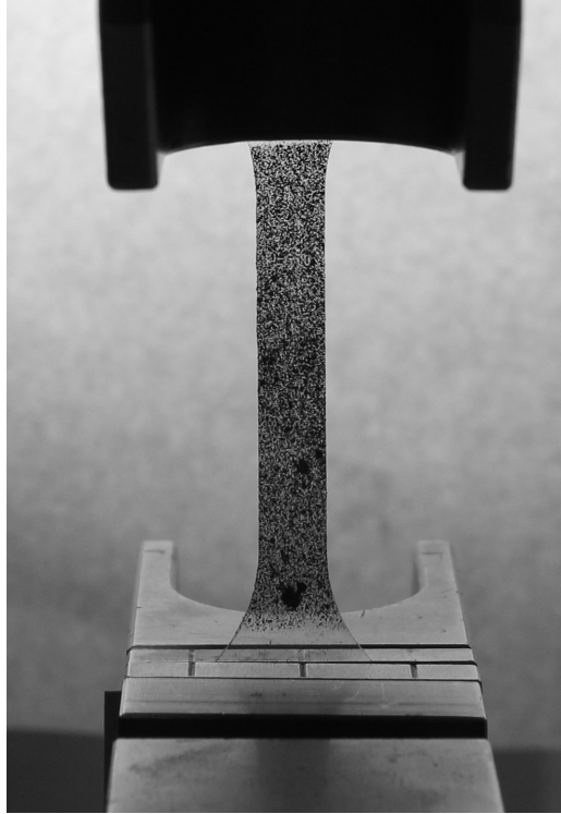
Figure 3.14: A LDPE test specimen that has been prepared with chalk paint.
