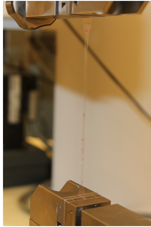
(b) A loaded and elongated polymer sample on a tensile test.
