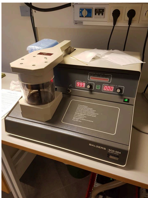
(a) The coater used for applying a conductive surface layer.
