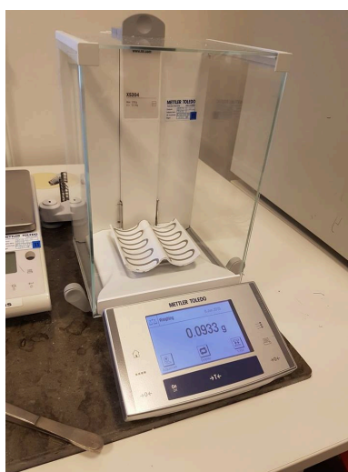
Figure 3.8: Product uptake measurement instrument with three significant digits.
