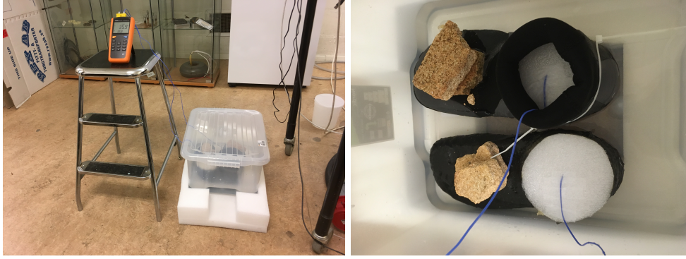
Figure 10: Experimental setup for thermal testing of the wetsuit-shoes.
