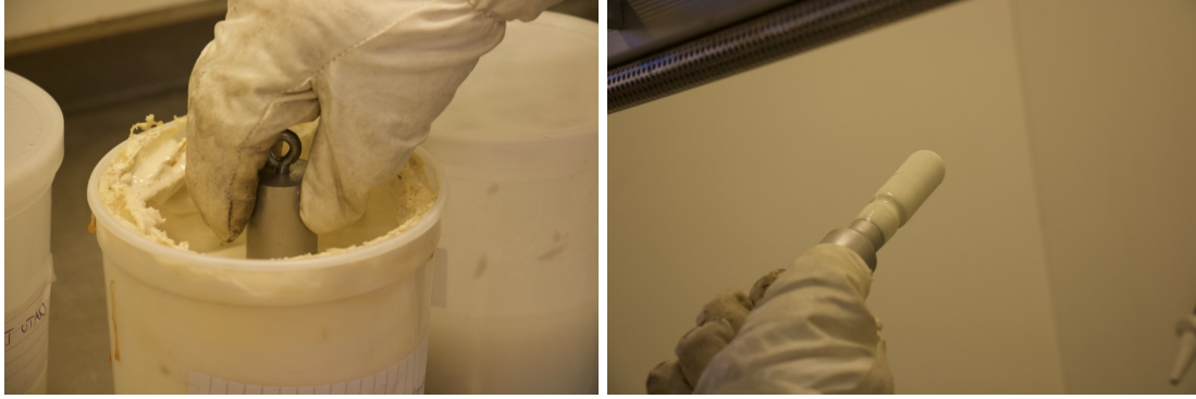
Figure 8: Images from the latex dipping process performed to produce the samples.
